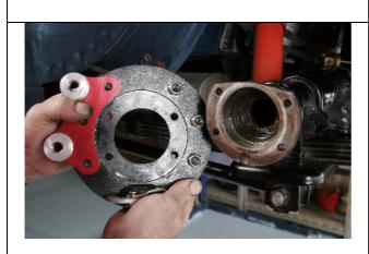
7. the spigot machined into the RRS mounting plate is clearly seen. Place the mounting plate onto the axle flange, making sure that it mounts flush to the axle housing by hand.
