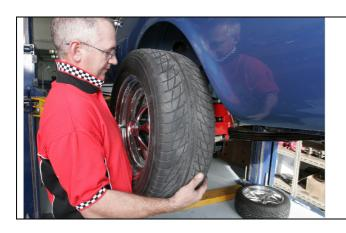
17. Fit the road wheels then check wheel nut tension. Follow normal brake bedding in procedures.
