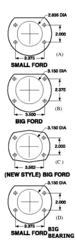
RRS Rear Brake Package kits are manufactured to bolt on without any modifications to standard Ford 8" or 9" axle housing with bearing diameter of 2.835 single row bearing or standard Ford 2.835 double row bearing. It is essential to check these requirements and specify when ordering that you have:
