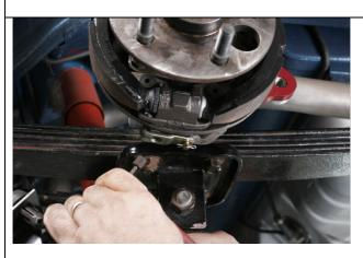
11.Fit factory cable end to RRS cable anchor. To make fitment easier, depress spring and hold with a pair of pliers. The RRS park brake mechanism will operate with all factory park brake cables regardless if it is foot or hand operated.
