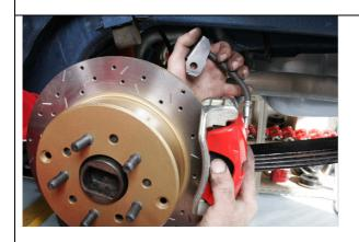
13. bolt the RRS caliper in place.
