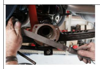
6. Remove axle assembly and backing plate. Check the axle seal and bearing for wear or leakage and replace if necessary. Check axle flange is free from burrs on the mounting face so that the RRS brake mounting plate fits squarely to the flange. Stamping flash is quite common on Ford axle housings and may require grinding or filing to neatly spigot into the CNC machined recess in the RRS brake mounting plate
